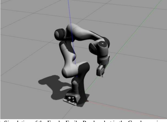
Fig.1. Simulation of the Franka Emika Panda robot in the Gazebo environment, showcasing its articulated structure and end-effector positioning. The setup illustrates the robot's capabilities for precision manipulation tasks within a virtual testing framework.
